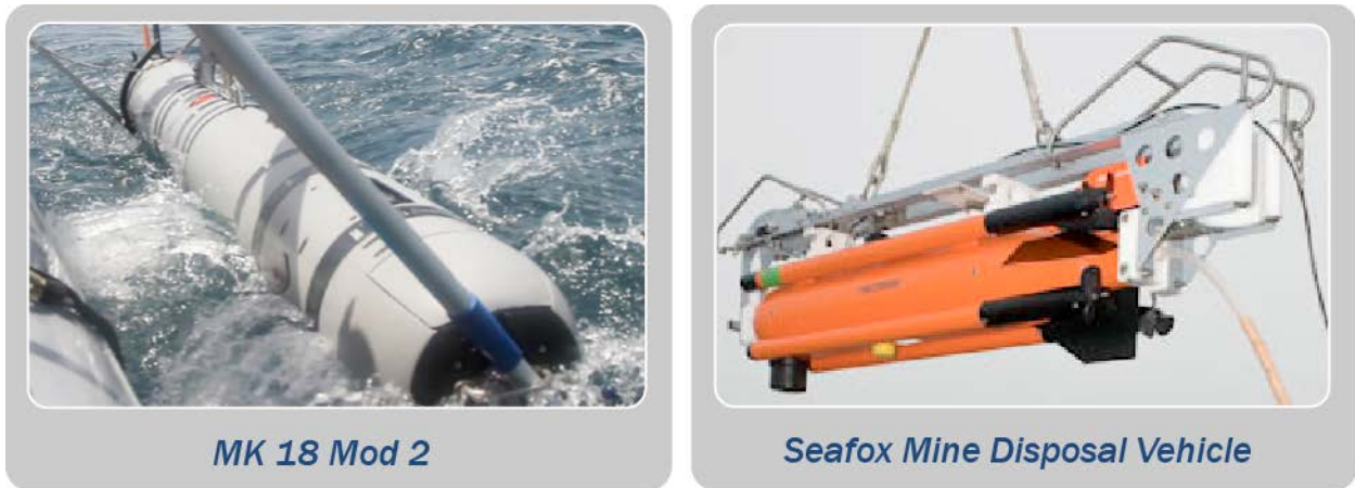
Figure 14 Current Mine countermeasure capabilities utilize two separate vehicles – an autonomous UUV for search and detection (left) and a vehicle remotely operated by a manned ship in the mine field for disposal (right).
