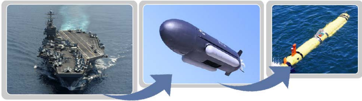
Figure 15 The cascading unmanned undersea vehicle concept deploys smaller UUVs with targeted payloads.
