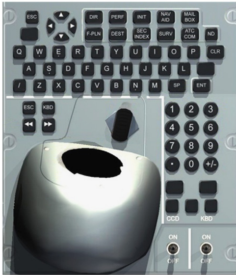
Fig. 1. KCCU (Keyboard Cursor Control Unit) for interactive cockpits taken from Aviation Week & Space Technology (September 27, 2004).
