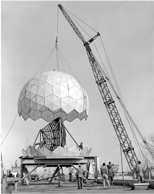
FIGURE B. On 25 February 1955, the radio-frequency (RF) loss of Lincoln Laboratory's second 31-ft-diameter rigid-space-frame radome was measured directly. The surface panels are irregular hexagons and pentagons. Improvements in fabrication technique made possible a weight reduction from 3900 lb (Figure A) to 2600 lb.
