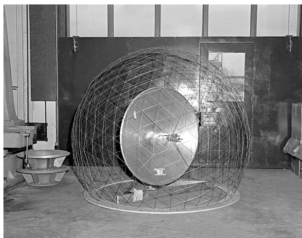
FIGURE E. Scale-model radome structure and antenna system under test to determine the far-field electromagnetic effects of having many metallic structural members in the near field of the antenna.
