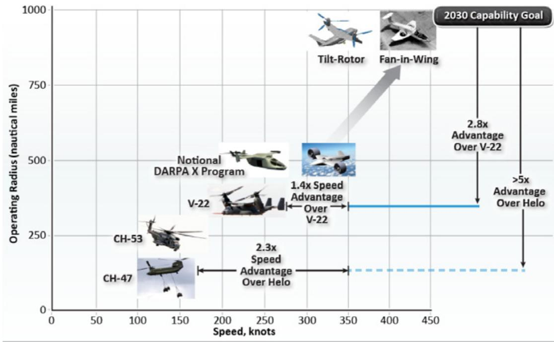
Figure 8 Operational Performance Capability for Enhanced Vertical Lift
